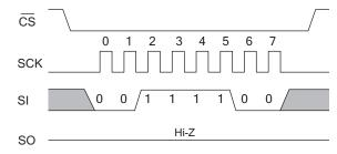
To issue this instruction, the device must be write enabled (WEN bit = '1'). The instruction is performed by transmitting the STORE opcode on the SI pin following the falling edge of  $\overline{CS}$ . The WEN
